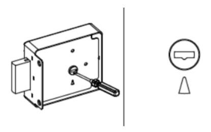
7) Now place the lock assembly from inside ensuring that connector strip enters into the slot at the back of the lock assembly. Fix it using the screws and check the functionality using keys.
