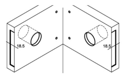
4) Place the cylinder with rose as shown and cut the strip as per the door thickness so that strip remains 8mm above the door surface.
