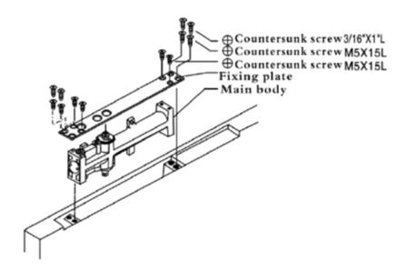
2) Fix the arm in the door frame to guide with the guide screw.
