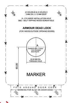
3) Make ø30MM through hole at point A using drill and cutter. From inside enlarge the hole to ø34mm X 3mm deep. Using chisel make 19 mm recess along marking on door edge as shown such that the lock flange lies flush with the door edge.
