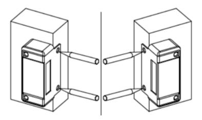
9) Make recess along this marking so that the flange of receptacle lies flush with the face of the door frame. Fix it using the receptacle screws as shown.
