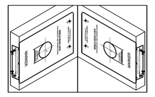
3) Make ø30MM through hole at point A using drill and cutter. From inside enlarge the hole to ø34mm X 3mm deep. Using chisel make 18.5 mm recess along marking on door edge as shown such that the lock flange lies flush with the door edge.
