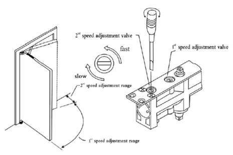
\* Open-Close angle (Stop angle is adjustable) adjustment method
