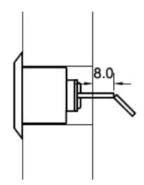
5) Now fix the cylinder using retainer plate on door as shown, so that QUBA logo on the cylinder is upright.
