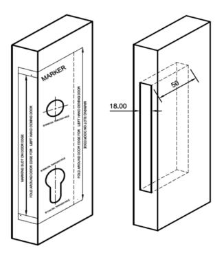
4) Now fix the lock body and handles using wooden screws, and Euro cylinder using cylinder fixing screw as shown.
