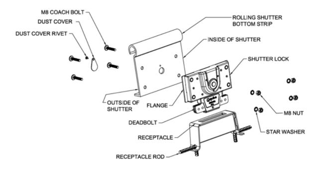
6) Fix the receptacle with concrete mixture using the lock in engaged condition provided lock is in the center position of the receptacle.
