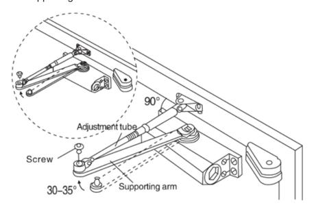
6) Now put the plastic cap and adjust the speed screws as per the requirement.
