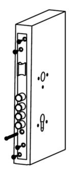
5) Now fix Rose Set handles using handle screws and Euro cylinder using cylinder fixing screw.
