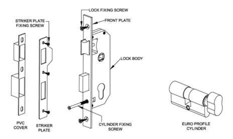
2) Cut the marker from the instruction manual given with the product, and fold along the dotted line as per the backset such as 20mm, 25mm & 30mm, and place on the door from inside as per the direction of the door opening as shown and punch the centers and mark the dotted lines along the thickness of the door. Mark horizontal lines on door thickness and mark two vertical lines 18mm apart from the middle of the door.
