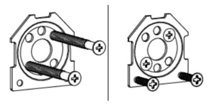
6) Place screw driver in the slot at the back side of the lock assembly and rotate it to align the mark on the spindle with the mark on the plate as shown.
