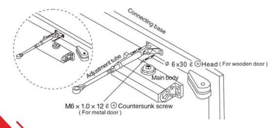
4) Install supporting arm on main body with screw
