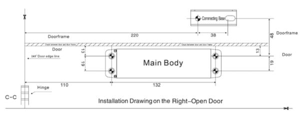
We will do installation on LH I/O door. Stick the marker from inside on right corner door and frame using adhesive tape as shown and punch the centers using punch center. Punch 4 holes on door and 2 holes on frame, and then drill holes of Ø 5 mm.
