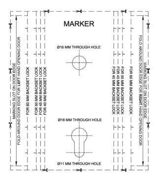
3) Make mortise slot of 18mm X 90 as shown using chisel and drill bits. Also make Ø16mm, Ø18mm and Ø11mm through hole from side of door for fixing handle shank and cylinder as shown.
