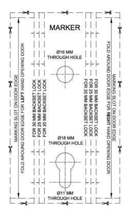
3) Make mortise slot of 18mm X 50 as shown using chisel and drill bits. Also make Ø16mm, Ø18mm and Ø11mm through hole from side of door for fixing handle shank and cylinder as shown.
