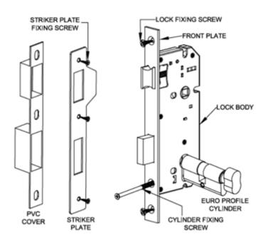
2) Cut the marker from the instruction manual given with the product, and fold along the dotted line as per the backset such as 40mm, 45mm & 50mm, and place on the door from inside as per the direction of the door opening as shown and punch the centers and mark the dotted lines along the thickness of the door. Mark horizontal lines on door thickness and mark two vertical lines 18mm apart from the middle of the door.
