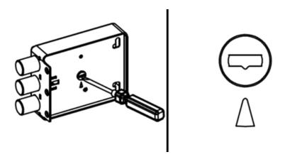
7) Now place the lock assembly from inside ensuring that connector strip enters into the slot at the back of the lock assembly. Fix it using the screws and check the functionality using keys.
