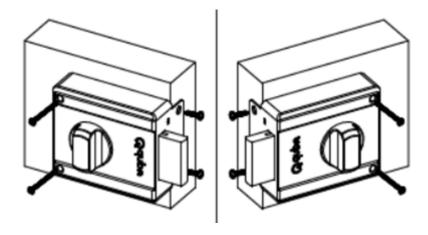
8) Now place the receptacle on the door frame from inside, slightly lower than the lock assembly to accommodate sag of the door. Mark its outline on the door edge.
