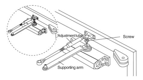
5) Regulate the adjustment arm to make it perpendicular to the door and fix the adjustment tube and supporting arm with screws
